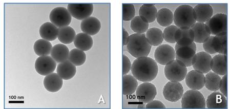
Figure 2 – TEM images of dense (A) and porous (B) γ-Fe<sub>2</sub>O<sub>3</sub>@SiO<sub>2</sub>-CaO core-shell nanoparticles
