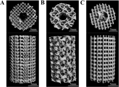
Figure 1. µCT scans of the three different scaffold geometries. (A) Lines, (B) Gyroid, and (C) Double Lines.
