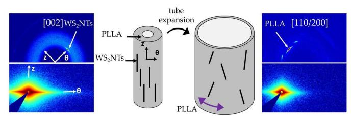
Figure 2 : WAXS (top) and SAXS (bottom) 2D patterns of PLLA/WS<sub>2</sub>NT tubesbefore and after tube expansion
