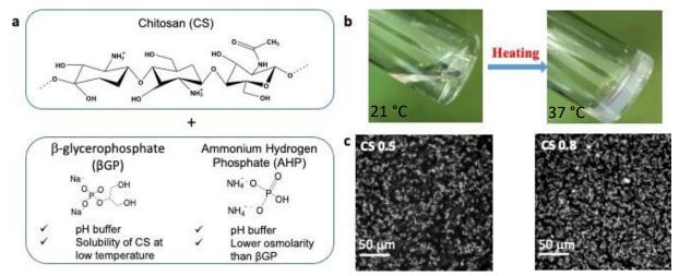
Figure 1. a) Composition of the studied thermosensitive system CS/ $\beta$ GP/AHP; b) Photographs showing the sol/gel transition; c) Confocal micrographs of fluorescently-labeled CS/ $\beta$ GP/AHP hydrogels having CS concentrations of 0.5 and 0.8 wt%.
