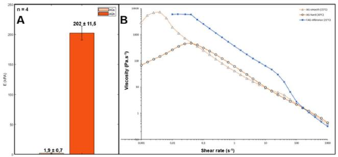
Figure 1: Rheological and mechanical characterizations of the hydrogel formulations. (A) Young Module measured on both AGs (0.5%Alg-2%Gel) and Agh (5%Alg-10%Gel) formulations in post crosslinking (1% CaCl2 for 30mn) after 24h at 37°C. Measurements performed by DMA compression tests, 8 mm geometry, with a DHR2 rheometer. (B) Study of the rheological profile of the 2 formulations AGs and AGh compared to the FAG reference (3d.FAB, Villeurbanne), measure by shear in sweep with a rheometer (DHR2, TA)
