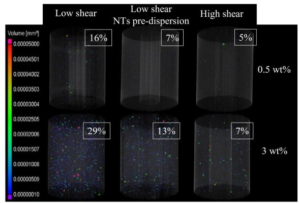
Figure 1: μ-CT images resulting from the inclusion analysis with the percentageof nanotubes mixed with the polymer that remain agglomerated
