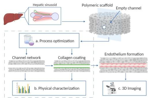
**Figure 1.** Schematic of the work presented here. The polymeric scaffolds containing an empty channel network have been optimized for both the fabrication and the coating steps (a) and then characterized (b). The constructs have been used as templates to form endothelium within the microchannels, subsequently imaged by different 3D high-resolution imaging techniques (c). Created with BioRender.com
